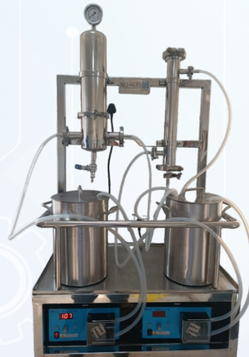
Tangential Flow Filtration
